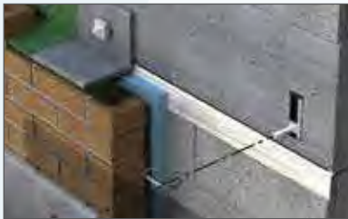
ST-4 Brick relief angle at concrete beam.
