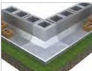
Outside Corner (Thru-Wall)
