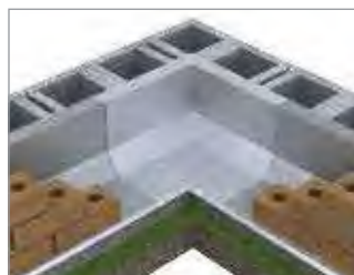
Inside Corner (Thru-Wall)
