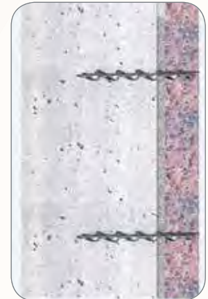
Dimensional Stone to Concrete or Masonry
