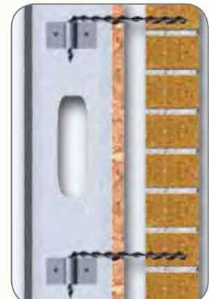
Interior: Steel Stud to Brick
